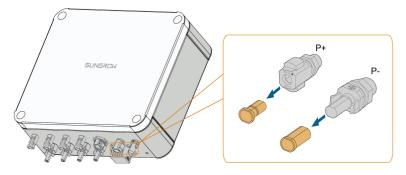
step 3 Plug the connectors into P+ and P- terminals.
