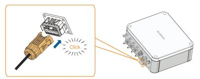
step 3 Pull cables outwards to confirm whether they are fastened firmly.
