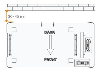
step 5 Place each battery module on top of the base.
