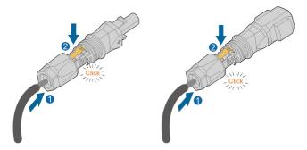
step 4 Push the insert into the sleeve and tighten the cable gland (torque 2 N·m).
