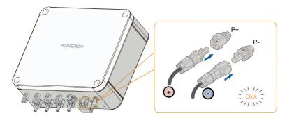
step 4 Ensure that the connectors are securely in place.
