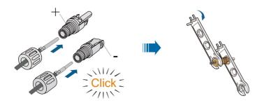
step 4 Check for polarity correctness.
