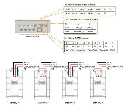
The COMM terminal of the battery is connected to the COM2 terminal of the combiner box. Signal cable 1 white and orange cable is used as BMS/CAN\_H1; signal cable 2 orange cable is used as BMS/CAN\_L1; signal cable 5 white and blue cable is used as BMS/CAN\_H2; and signal cable 6 green cable is used as BMS/CAN\_L2.
