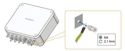
step 3 Apply paint to the grounding terminal to ensure corrosion resistance.
