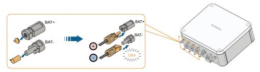
step 2 Seal the unused Battery terminals with the terminal caps.
