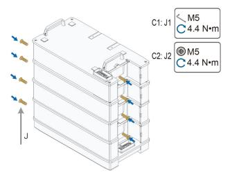
step 7 Connect the switch gear to the base.
