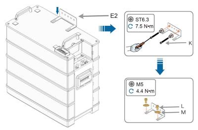
The bracket is mounted on the top battery module.
