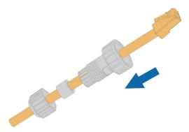
step 4 Tighten the swivel nut.
