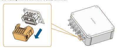
step 2 Insert the COM2 connector into **COM2** terminal on the bottom of the combiner box until there is an audible click.
