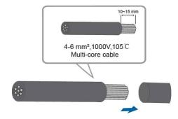
step 2 Pry the connection open and pull the sleeve and the insert apart.
