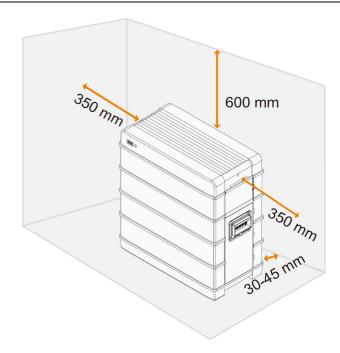
• In case of multiple batteries, reserve specific clearance between the batteries.
